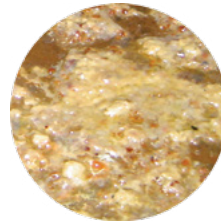
Varnish deposits on reservoir floor (Plated)
