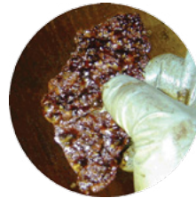
Varnish can be hard and brittle (Lacquer)
