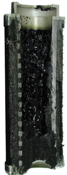
Filter element cross section (Lacquer Varnish Deposits, Support Tube)
