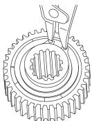
1. Remove the snap ring and sprag bushing retainer from one end only.
