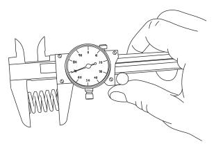
Check brake spring free length; minimum free length is 15/16 in. (23.8 mm). Check springs for any sign of cracking or failure. If a brake spring must be replaced for any reason, then ALL brake springs must be replaced.
