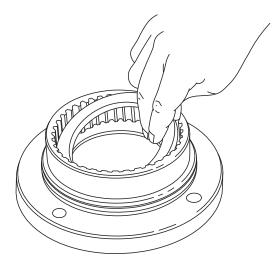
2. Install a brake spacer into the motor support. (Not required with lobed discs.)
