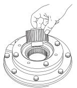
3. Remove the brake clutch assembly from the motor support.
