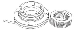
New lobed steel brake separator plates and motor support. Note groove on outside diameter of motor support.
