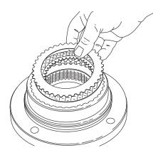
3. Insert first, a steel brake disc against the spacer followed by a friction brake disc then alternate steel and friction discs until seven (7) friction and eight (8) steel discs have been installed. Finish with a steel brake disc on top.
