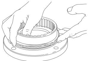
1. Begin assembly by placing motor support on workbench with motor mounting surface down. Install new O-ring and back-up ring as shown.
