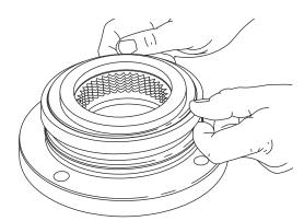
6. Lubricate the brake piston seal and motor support sealing surface with petroleum jelly or hydraulic oil. Install new piston seal to motor support, seal lip down.
