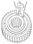
4. Remove the snap ring and sprag bushing retainer from one end only of the brake clutch assembly.
