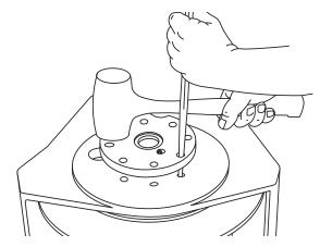
3. Center the drum in the opening of the base. Lubricate the bearing support with petroleum jelly or gear oil and install in base and drum.
