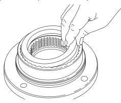
4. Install the remaining brake spacer on top of the last steel brake disc. (This is the only spacer used with lobed discs, except on some of the 67:1 ratio units with the 1.3 displacement motors, two of the spacers are stacked on the brake discs.)
