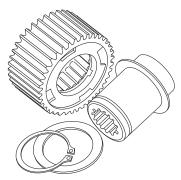
5. Pull the inner race out. Examine the race for scoring, wear or indentations caused by the sprag cams. If the inner race is not completely smooth, the assembly should be replaced.
