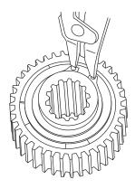
6. Turn the assembly over with the snap ring down. Install the second retainer and snap ring. Make certain the snap ring is seated in the groove properly.
