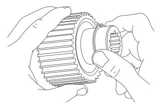
Slide the inner race through the bushings and sprag clutch (the race will have to be rotated in the freewheeling direction to start it through the sprag clutch). If the inner race will not go through the bushings, the bushings have probably been damaged and should be replaced.
