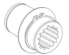
4. Next, install a sprag bushing retainer, then a snap ring on the inner race. Be sure the snap ring is seated in the snap ring groove.
