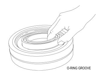
Install a new bearing in the drum closure as required. Use sealant on the outside surface of the oil seal. Install with spring side of the seal toward bearing, using a flat plate to avoid distortion.
