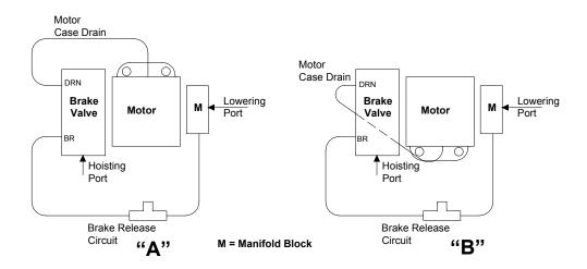
**NOTE:** Only BG6A and BG6B hoists equipped with gear motors and Braden cast brake valves are capable of being configured for opposite, or underwound drum rotation.
