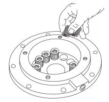
3. Remove the brake springs.
