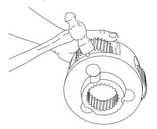
3. Carefully align the pin hole in the carrier with the hole in the planet gear shaft and drive the roll pin into place. Always use NEW roll pins. When properly positioned, 50% of the roll pin will engage the planet gear shaft and 50% will remain in the planet carrier.
