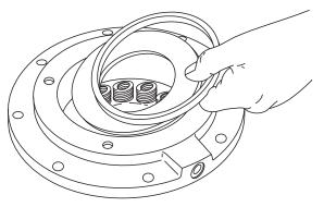
2. Remove the piston back-up ring and pressure plate.
