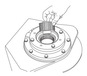
12. Install the brake clutch assembly.
