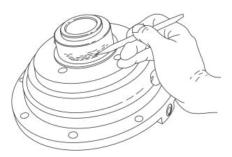
2. Check oil seal and bearing surfaces on brake cylinder for damage or wear.
