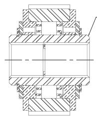
Assemble so that inner race freewheels in the opposite direction of desired cable drum rotation for hoisting when viewed from motor side.
