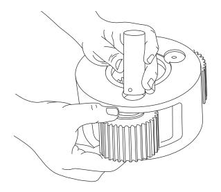
2. Insert two (2) bearings and a bearing spacer into a gear with the spacer between the bearings. Place a thrust washer on each side of the gear and position in a carrier opening. Slide the shaft through the carrier, thrust washer, bearing-gear sub-assembly and remaining thrust washer.
