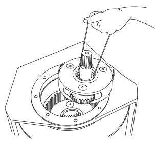
8. Install the primary planet carrier, meshing the planet gears with the ring gear and the planet housing with the output sun gear.
